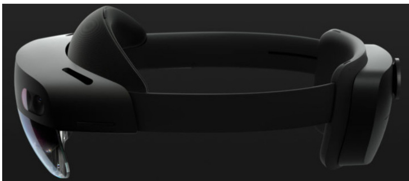
Figure 3: A diagram of the Microsoft HoloLens 2 AR headset to be embedded with the developed software platform. Clinicians will be wearing these during procedures to visualise the predicted tumour locations onto patients directly. This image is from the Microsoft News Center Image Gallery.
