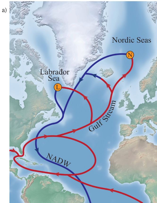
Figure 1: (a) The North Atlantic component of the AMOC with deep water formation sites at L and N in the Labrador and Nordic seas. The background is generated with the software from [8] and ocean currents are illustrated following from [10]. (b) Two-box model for temperature and salinity in the surface and deepwater layers at sites L and N.
