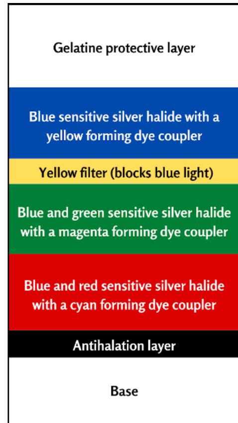
The 7 layers of colour negative film.
